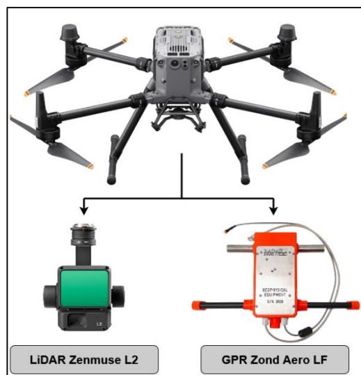
Fig. 7. Conceptual design of a modular unmanned aerial vehicle for engineer reconnaissance of a water obstacle
