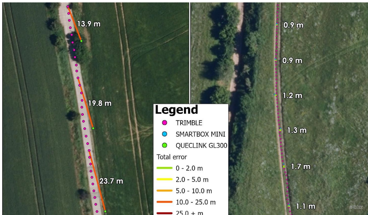
Fig. 1. Visual comparison of trajectory recording during pedestrian movement in open terrain. Left: Legacy tracker (Queclink GL300) exhibiting massive along-track latency and corner-cutting. Right: New generation tracker (Smartbox Mini) demonstrating elimination of latency and sub-meter positional accuracy.
