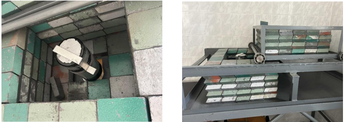
Fig. 1. The pictures of the scintillator with the photomultiplier (the middle of the left picture) and neutron source shielding (right picture).
