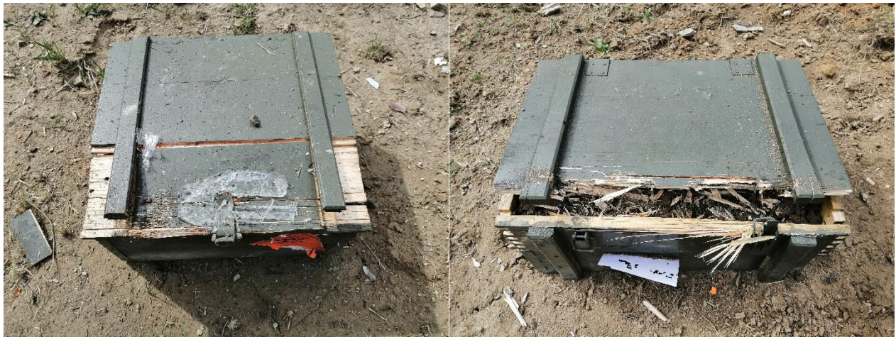
Fig. 4 Comparison of detonation effects: water-backed charge with a pushing effect (left) and standard fragmentation effect (right)
