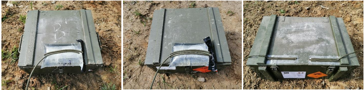
Fig. 2 Assembly of water charges consisting of two and three detonating cord segments, including the arrangement of the detonating cord initiation network (left and middle) and standard charge without water (right)
