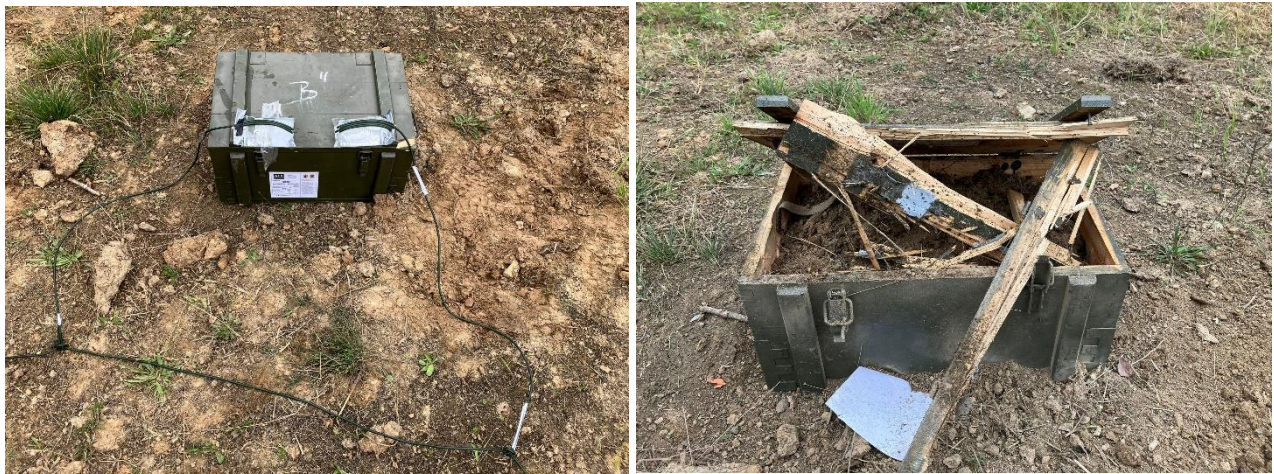
Fig. 1 Assembly of water charges consisting of three and four detonating cord segments, including the arrangement of the detonating cord initiation network (left) and effect of detonation (right)
