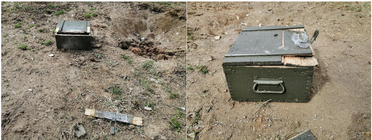
Fig. 3 Effect of detonation of water charges consisting of two (left) and three (right) detonating cord segments
