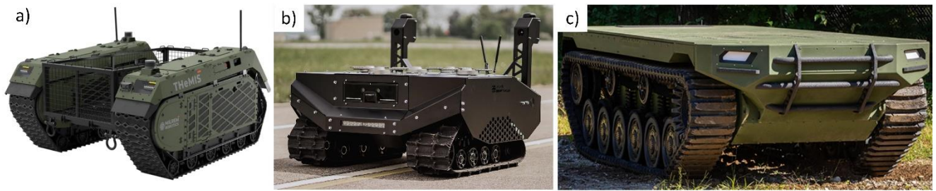
Fig. 2. Analyzed UGVs with tracked running gear system: a) Themis; b) Gereon RCS; c) Ripsaw M3 [12 - 14]
