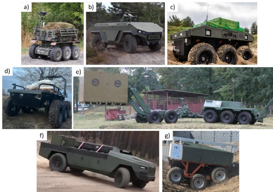
Fig. 1. Analyzed UGVs with wheeled running gear system: a) IBIS; b) Hunter; c) UNL; d) Ratel X e) Boguś; f) Protector; g) ExMot. [6 - 11]
