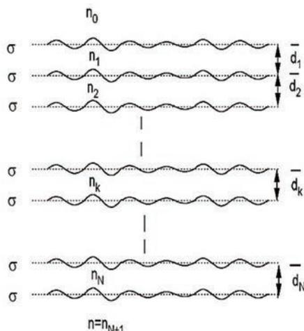
Fig. 1. The system of thin films with identically rough boundaries
