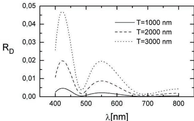
Fig. 3. Spectral dependences of the diffuse reflectance of the single  $\text{TiO}_2$  layer on glass for various values of  $T$ .
