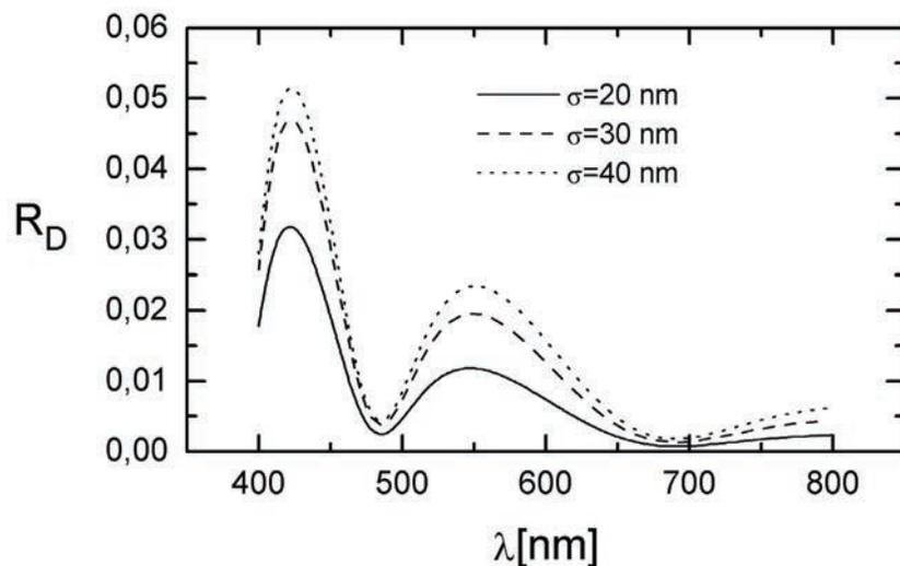
Fig. 2. Spectral dependences of the diffuse reflectance of the single  $\text{TiO}_2$  layer on glass for various values of  $\sigma$ .
