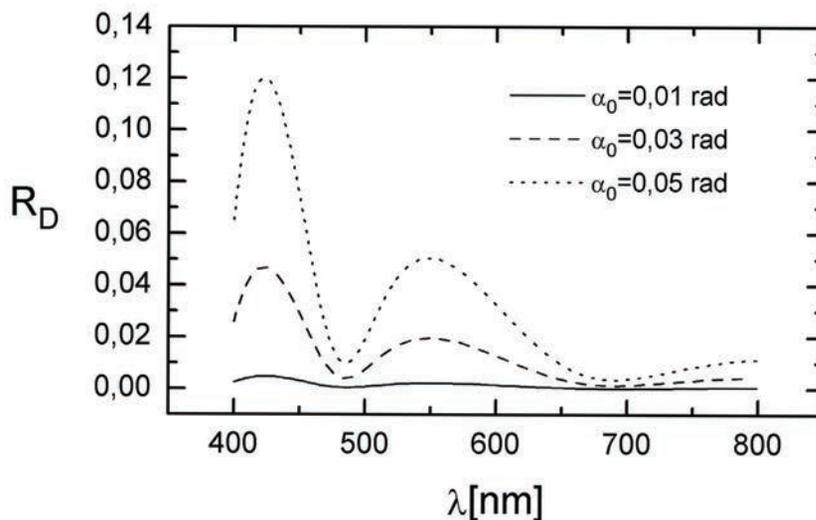
Fig. 4. Spectral dependences of the diffuse reflectance of the single  $\text{TiO}_2$  layer on glass for various values of  $\alpha_0$ .
